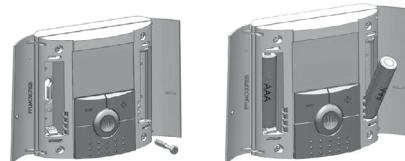
Open the two side's covers and Insert the 2 AAA Alkaline supplied batteries (or remove the small protection sticker if the batteries are already installed in the compartment).
