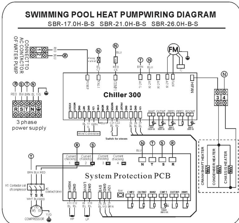
Note: cranks heaters marked in diagram are optional parts according to customer request!
