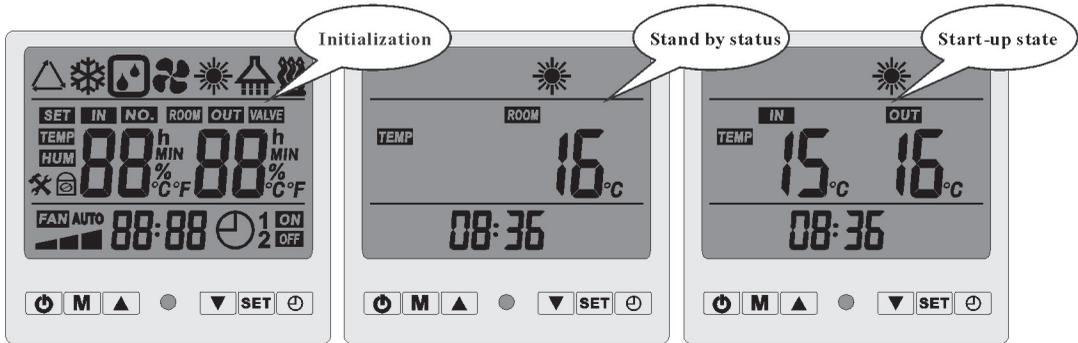
Remarks: Standby status means the unit is connected with electricity but not running.
