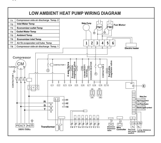
Note: crank heaters marked in diagram are optional parts according to customer request!
