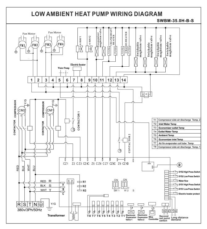
Note: crank heaters marked in diagram are optional parts according to customer request!
